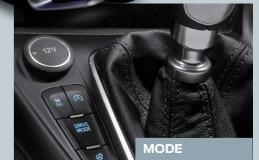
The Drive Mode control switch is located alongside the gear lever, where it can be located quickly and easily by the driver.
